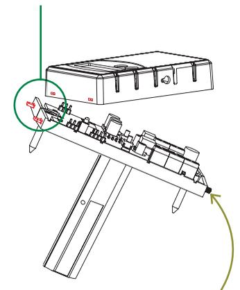
Once lid closed, insert set-screws to lock enclosure. Requires 1/16" Allen Wrench
